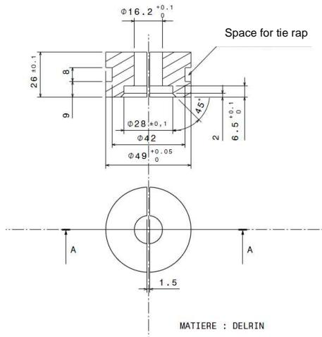
This additional bump stop, machined in Delrin, must be fit between the bottom part (part connected to the reservoir) of the damper and the elastomer bump stop, the face with the counter bore in contact with the bottom part of the damper. The parts must be fixed together with tie rap and metallic wires in the dedicated space.
