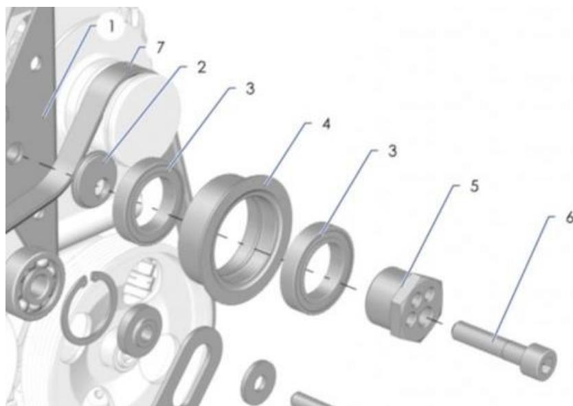
As a matter of fact, **the correct bearings have green plastic sealing rings while those which are not correct have black plastic sealing rings.**
