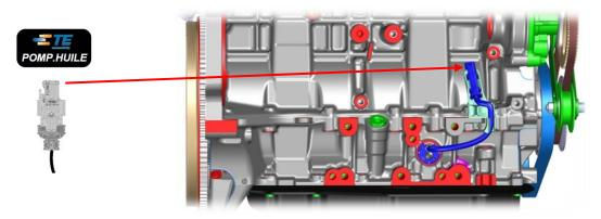
We advise you to control the state of the solenoid valve as well as the state of the engine loom before connecting them together.
