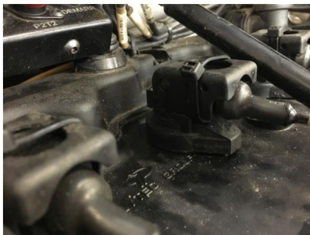
Wrong seal position (to the front)
