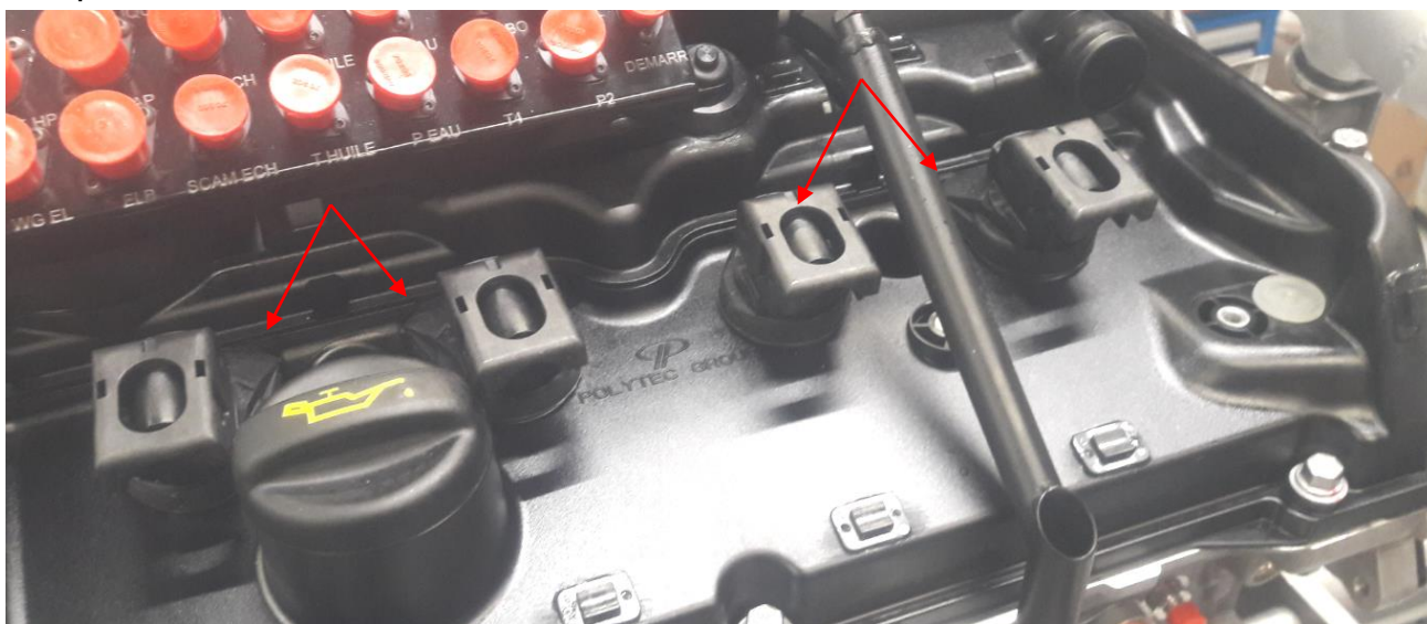
Correct seals position (backwards, into the notches)
