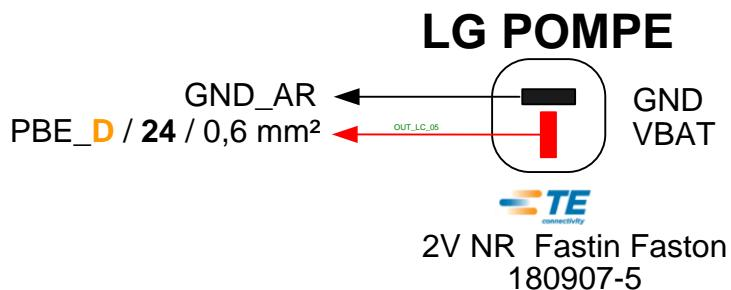
A new release of the chassis loom correcting this inversion will be deployed (release P) and the current looms (release N) that will be corrected will have a green sticker at the windscreen washer connector.
