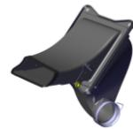
To avoid any water intrusion through the airbox during parking under the rain or washing, we recommend you to cut the lower side of the upper airbox (904481078D) as picture below (thickness = 1 to 2mm):
