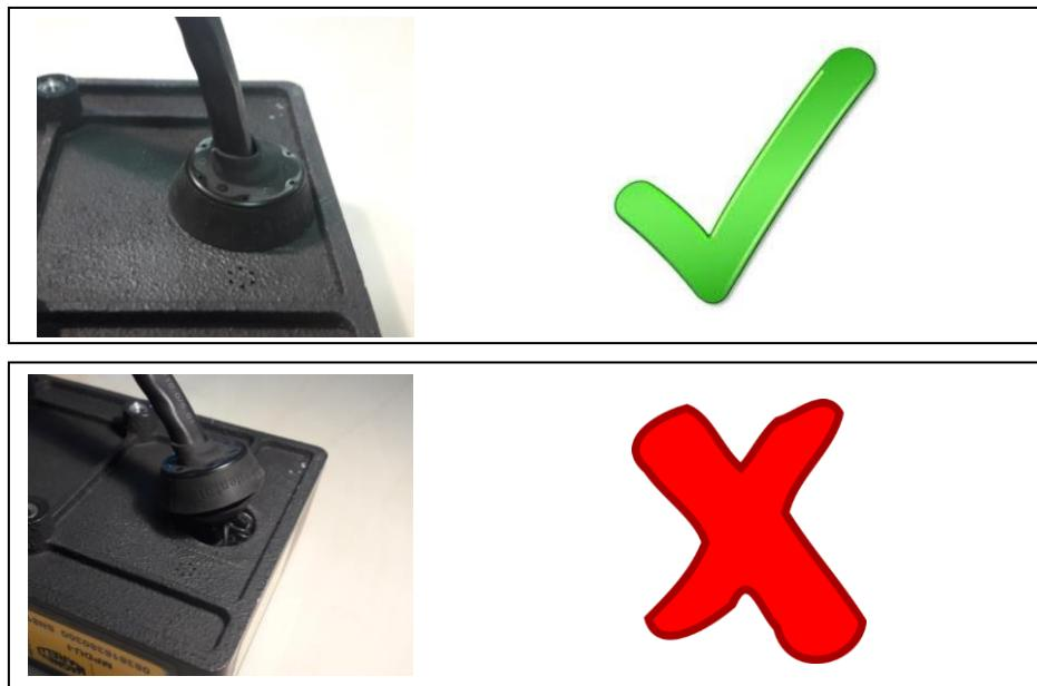
To lock the grommet, the 2 lugs (diametraly opposed) must be engaged inside the housing by pushing to the center of the grommet. A small noise can be heard when correctly placed (do not use tools to put it in place).
