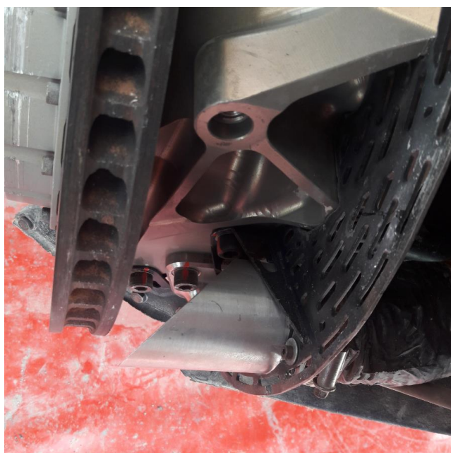
Rear cooling duct fitting
