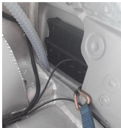
Rear fan loom through the chassis scoop
