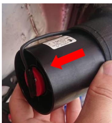
Blowing way (fine mesh is missing)
