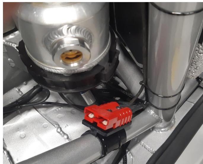
The drilling drawing for the new master relay position is available at the end of this document. We advise you to use some thread rivet nuts (M5) to fit the master relay to the chassis.
