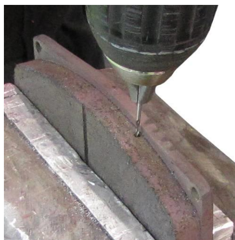
Example of TCK sensor fitting and hole drilling (taken from DS3R3 as no picture available for C3Rally2)
