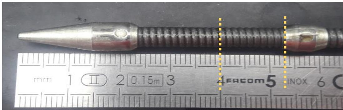
Max level (under the ball) is at 53mm, min level is at 40mm
