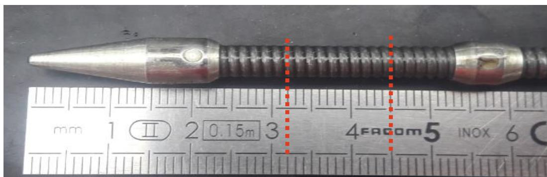
Max level is at 45mm (8mm under the ball), min level is at 32mm
