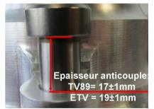
The guide diameter of the two fixation holes on your anti-torque must be  $\emptyset$ 12 H8. The tapping inside the crankcase of the gearbox is M10x1,5 reinforced by replaceable helicoils (helicoils reference: 212000007)
