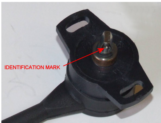
Typical hall-effect gear position sensor
