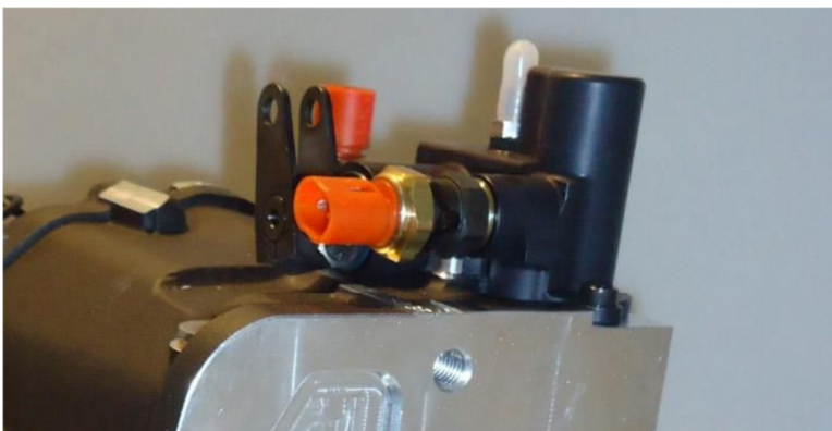
Built-in cut switch – Sadev SCL82
