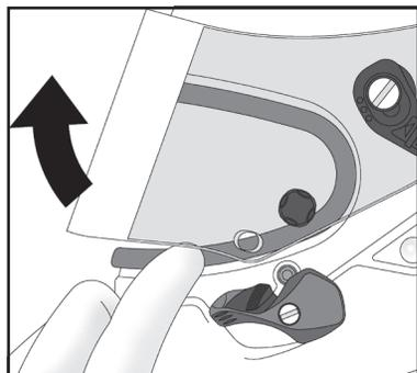
To close the shield, push down the shield until it is locked in place.
