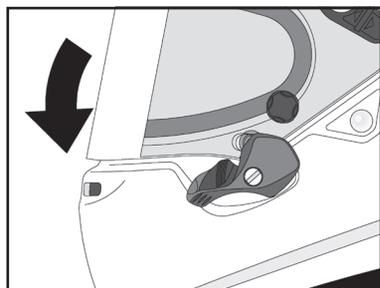
To remove the shield, remove screws, washers and guides from the helmet. To replace, position the shield in place and install guides, washers and screws as illustrated.
