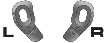
Tear-Off posts are standard equipment. To install the Tear-Off, some Tear-Offs come with protective film on one or both sides. Be sure to remove any films that may be present. Slip the hole of the shorter end over the right shield post. Lay the Tear-Off across the shield and slip the other hole over the left shield post.
