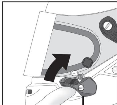
Then raise the shield. The shield can only be opened when the lock system has been so released.
