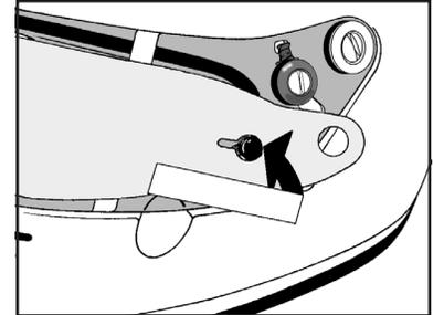
Arai Tear-Off posts are eccentrically mounted so as to be adjustable to better accept looser or tighter Tear-Offs. Adjust both posts by rotating them so that the Tear-Off is taut across the shield but not too tight so as to rip or distort the Tear-Off.
