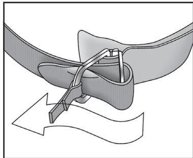
A D-ring release tab is provided to make loosening of the strap easier, simply pull as illustrated.
