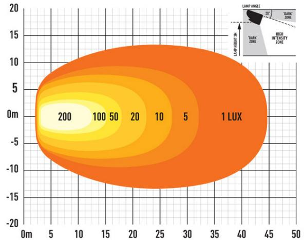
Generated from BSI lamp photometric test data: on road measurement data
