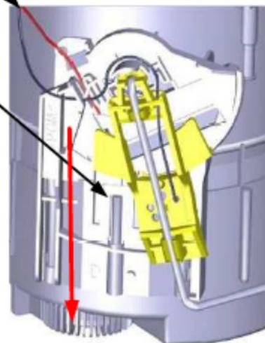
The fuel pump 904 244 508 A is the block DPR reference gauge 96 744 669 80 which we have removed the gauge assembly
